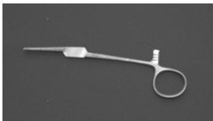
Forging (de-burred and annealed)
