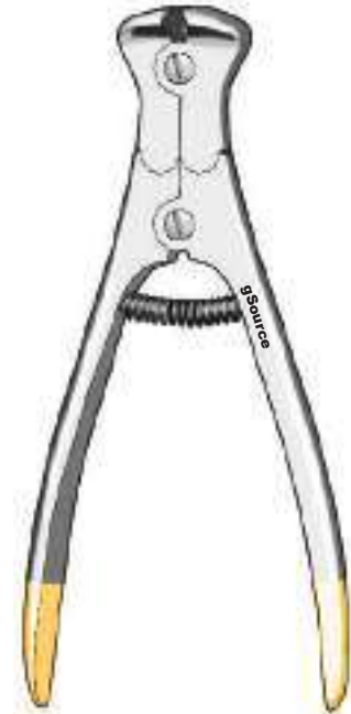
gS 83.7512 6" Wire End Cutter DA TC inserts max cap 1.6mm [.062"]
