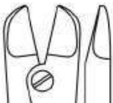
gS 83.7228 6 1/2" Wire Side Cutter DA Angled TC inserts max cap 1.6mm [.062"]
